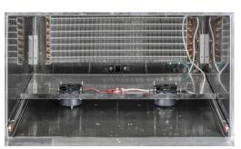
The fans are hard-wired, but the panel can be rested on the runners whilst servicing.
