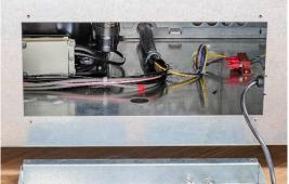
Removable panels, on the right and rear of the cabinet, provide further access to the refrigeration equipment.
