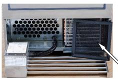
The pre-filter should be removed and cleaned regularly.
