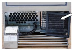
The cabinet is fitted with a removable filter, which will catch most of the dust and fluff, before it reaches the condenser radiator.
